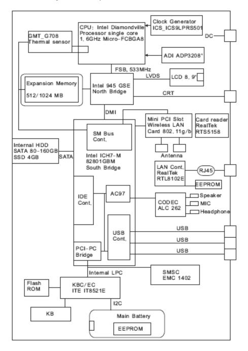
Figure 1-4 System Unit Block Diagram
